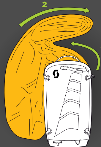
PUSH THE AIRBAG TOWARDS THE LEFT AND PUSH THE UPPER PART TOWARDS THE RIGHT. LEFT HAS TO OVERLAY THE RIGHT PART
